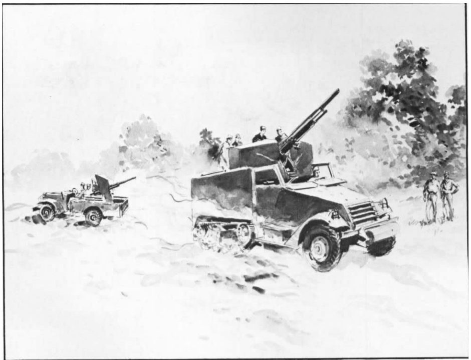
Sketch by Vernon H. Bailey, Navy Art Collection Maneuvering at the Marine Barracks, New River, North Carolina in 1942 is an armored half-tracked mounting a 75mm gun, M1897A4, as well as a 3/4-ton truck carrying a 37mm antitank gun. Later in the war a jeep would pull this weapon.
