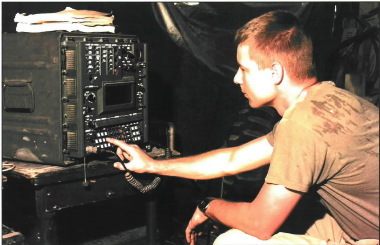
U.S. Air Force SSgt Rick Robinson of the 52d Combat Communications Squadron adjusts an SB3865 tactical telephone switch at the U.S. Embassy in Mogadishu. The squadron provided communications support for the Air Force's Air Mobility element.
