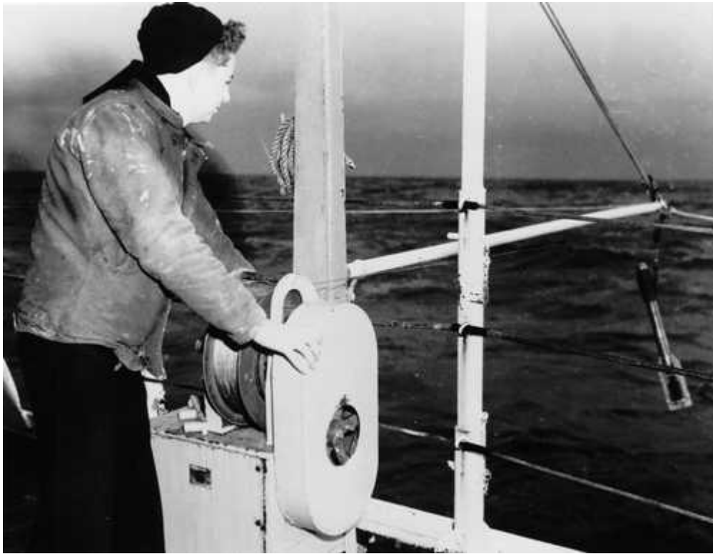
A Coast Guard crewman readies a bathythermograph. The device recorded sea water temperature to a depth of 450 feet.
