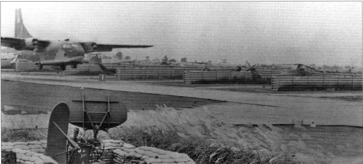
A C-123 Provider becomes the first fixed-wing aircraft to land on the improved airfield at Khe Sanh Combat Base. In the background are several revetted helicopters, and in the foreground is the Precision Approach Radar used to guide aircraft in to land during low visibility conditions.
