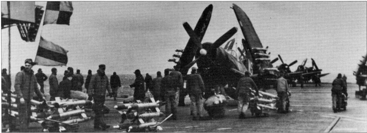
Deck crew loading rockets on the wings of F4U-4 Corsairs aboard the carrier Badoeng Strait off Korea in September 1950. Although a holdover from World War II, the relatively low-speed, long-endurance, and durable Corsair proved to be an indispensable CAS aircraft, most notably in the early stages of the war. Corsairs provided critical support for the defense of the Pusan Perimeter and in the extremely dense weather that complicated operations in the Chosin Reservoir.
