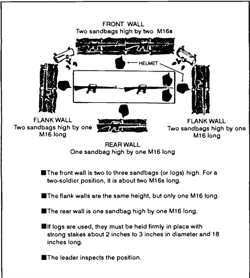
Figure 2-45. Stage 2, preparation of a fighting position.
