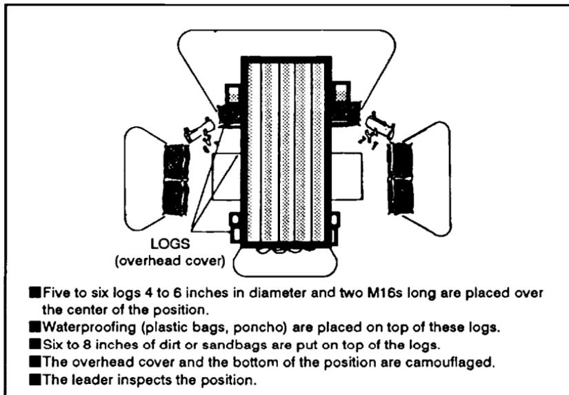
Figure 2-47. Stage 4, preparation of a fighting position.
