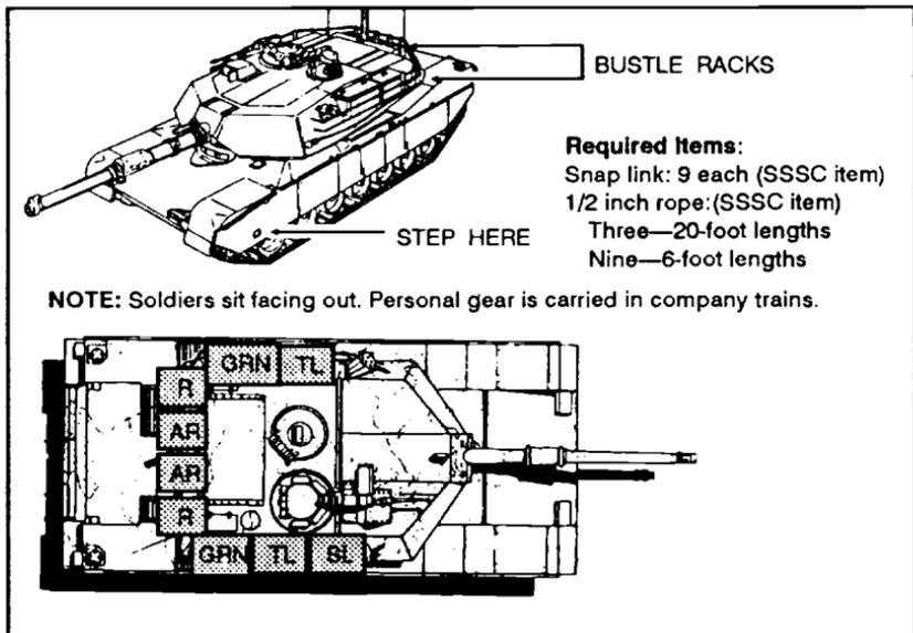
Figure 2-74. Mounting and riding arrangements on an M1.
