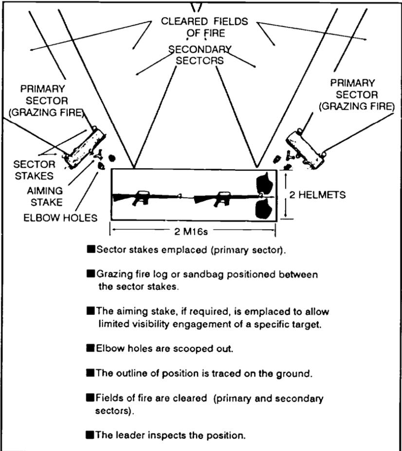
Figure 2-44. Stage 1, preparations of a fighting position.
