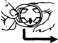
**4** Screw detonator into detonator well
