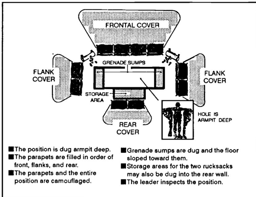
Figure 2-46. Stage 3, preparation of fighting position.
